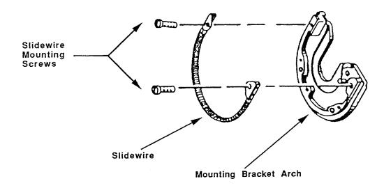
*Caution:* Make certain that the slidewire is as close to the mounting bracket arch as possible by pushing the slidewire against the mounting bracket arch when tightening the mounting screws.
